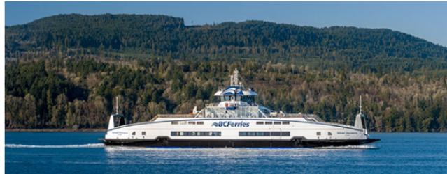
The Island Class are battery-equipped ships designed for full electric operation. The ships are fitted with hybrid technology that bridges the gap until shore charging infrastructure becomes available. From the exterior details to the engines, the design of the new vessels reduces underwater radiated noise, lowers emissions and improves the customer experience on board.
